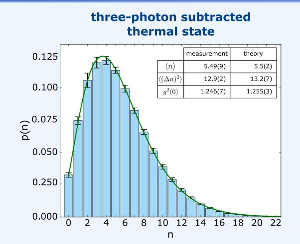
Multiple-photon subtraction from thermal state was implemented by using a low-reflectivity beam splitter (R = 5%, half-wave plate + polarizing beam splitter). Reflected photons are detected via a reconfigurable multichannel detector (multiple commercial on-off detectors). When many-fold coincidence is detected by the multichannel detector in the reflected port, the heralded optical signal in the transmitted port is analyzed by PNRD [2].
