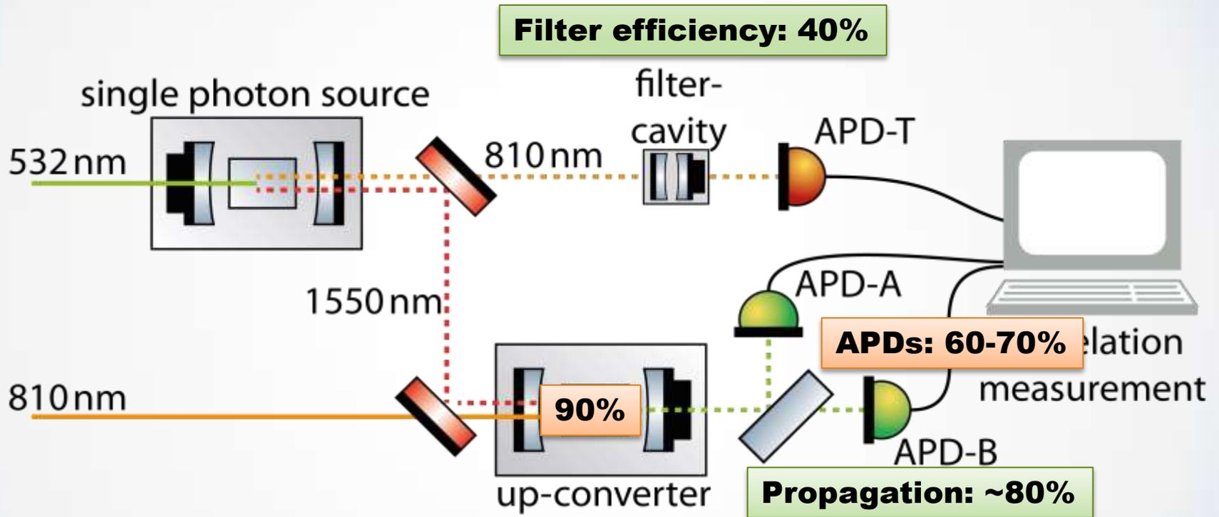
**Additional filtering and new components would increase the detection efficiency to about 60%!**
