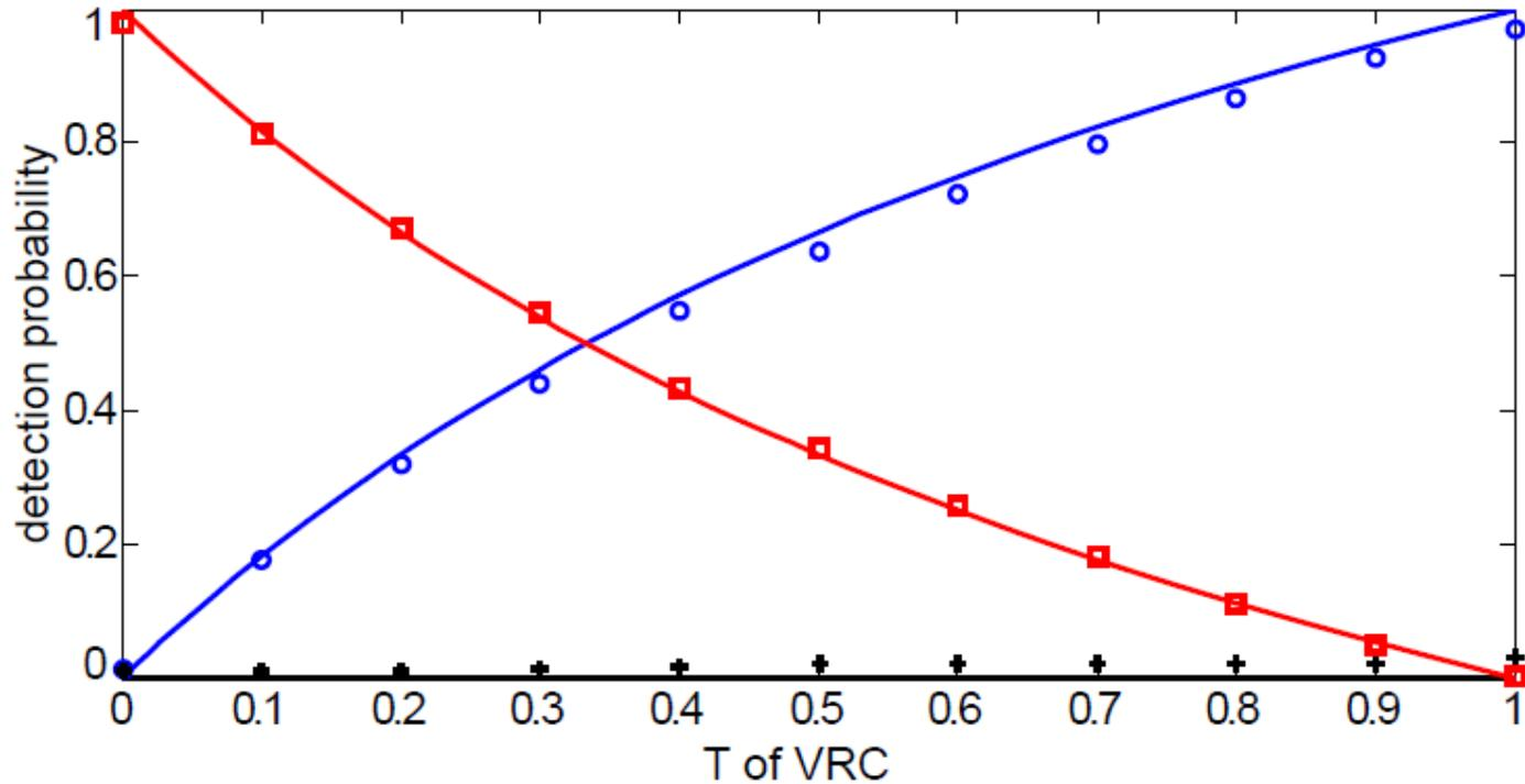
FIG. 4: Unambiguous discrimination of quantum measurements. The probabilities  $P_S$  (blue circles),  $P_I$  (red squares), and  $P_E$  (black crosses) are plotted as functions of the VRC splitting ratio  $T$ . The lines represent theoretical predictions.
