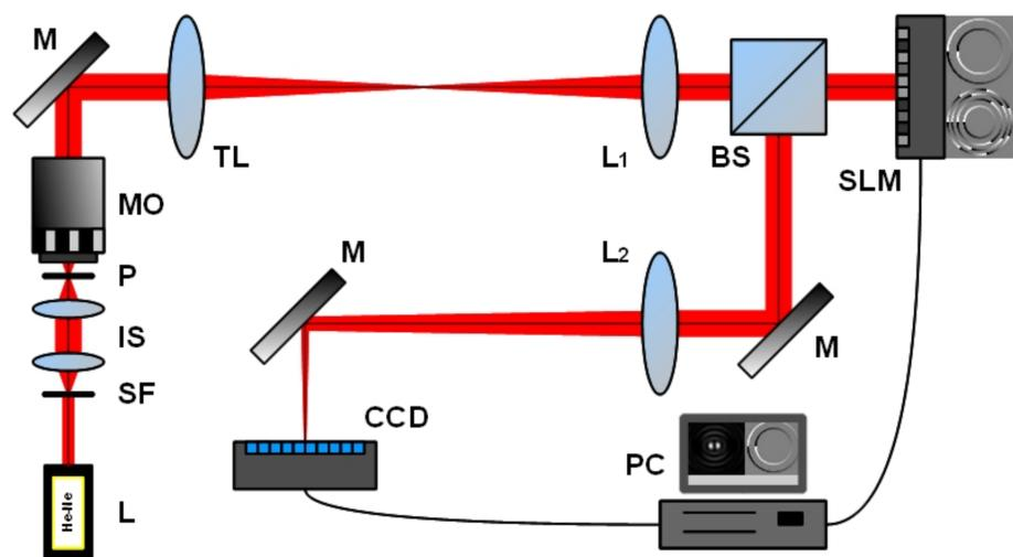
L – laser (632.8nm, 20mW), SF – spatial filter, IS – illumination system, P – pinhole (2μm), MO – microscope objective (Newport 20x, NA = 0.4, fo = 9mm), M – mirror, TL – tube lens (ft = 200mm), L1 – lens (f1 = 200mm), BS – beam splitter, SLM – spatial light modulator (Hamamatsu X10468, 600x800px), L2 – lens (f2 = 400mm), CCD camera (Olympus F-view II).
