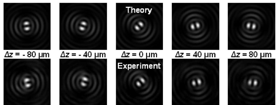
Spherical aberration causes constant additional rotation only and its effect can be completely eliminated in axial localization.
