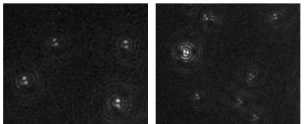
Vortex self-imaging was successfully applied to 3D localization of freely moving 1 μm polystyrene beads.
