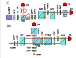
NLC - nonlinear crystal, SMF - single-mode fiber, BD aicite beam lispiacer, PPB9 partially beam splitter, PBS - polarizing beam splitter, HWP - half-wave plate, QWP - quarter-wave pate, D - singlephoton detector, DB - detection block consisting of a HWP, QWP, PBS and two single photon detectors.
