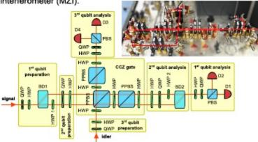
BD - calcite beam displacer, PPBS - partially polarizing beam splitter with transmittances TV = 1/3 and TH = 1, PBS - polarizing beam splitter, HWP - half-wave plate, QWP - quarter-wave plate, D - single-photon detector.
