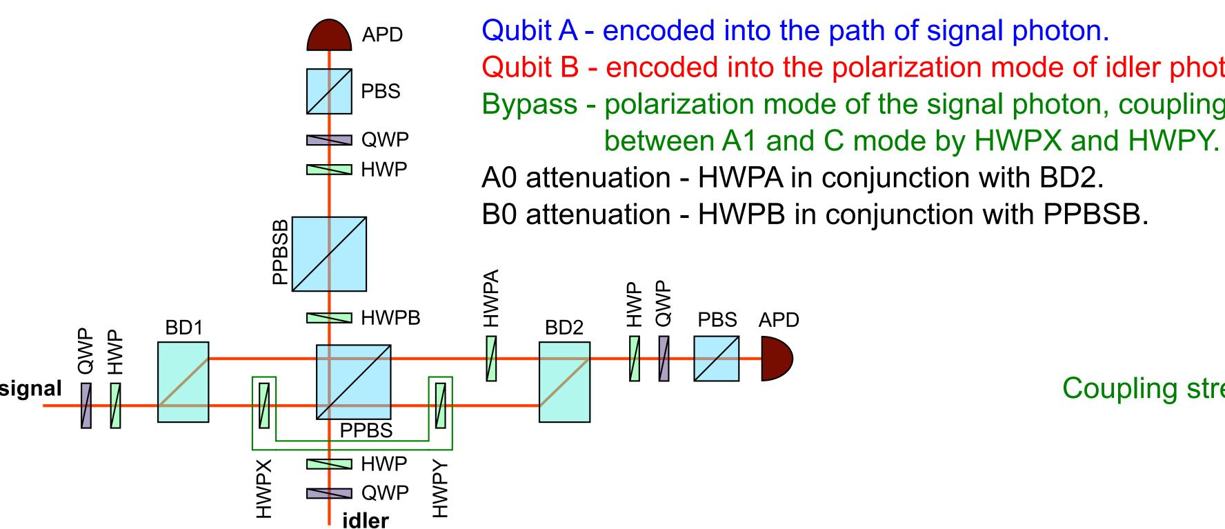
Qubit B - encoded into the polarization mode of idler photon. Bypass - polarization mode of the signal photon, coupling
