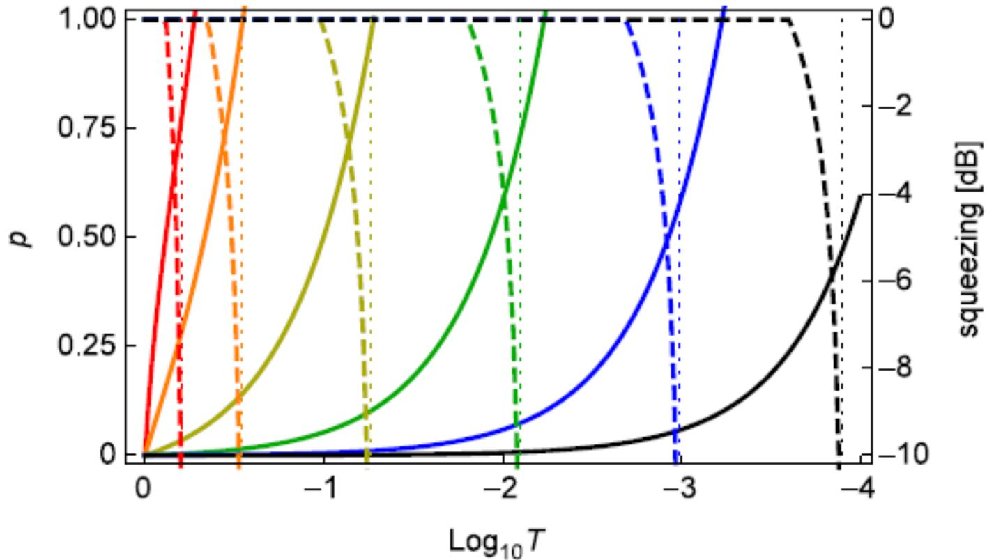
Requirements on nonclassicality of the sources for CV and DV in noisy channels
