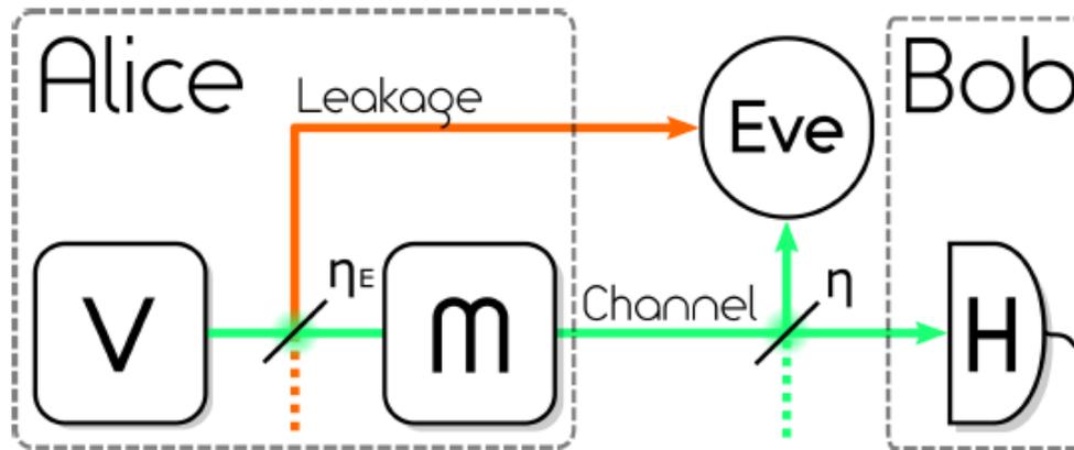
Lossy side channel prior to state modulation
