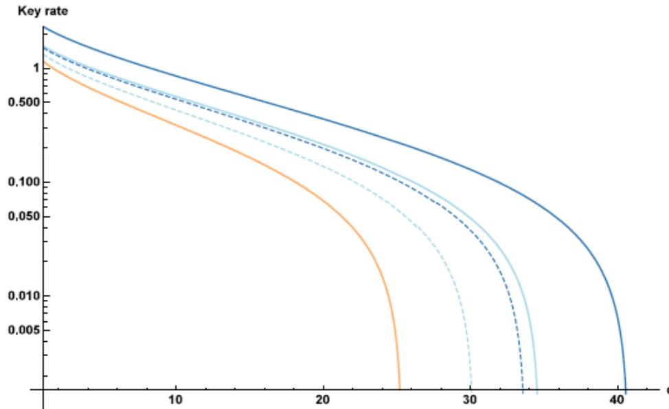
Key rate vs distance without (solid lines) and with a 50% pre-modulation side channel.
