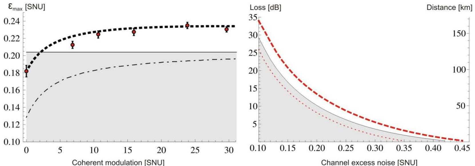
Maximum tolerable channel noise versus modulation (left) and maximum tolerable noise for given channel noise (right) for optimized coherent-state protocol (grey area) and squeezed-state (theory dashed lines + experimental points)
