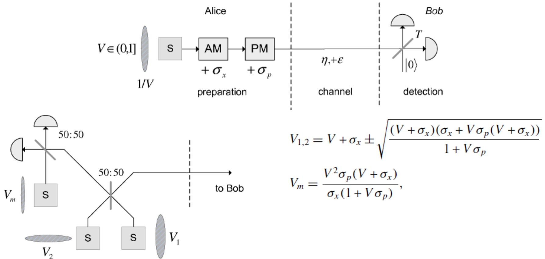
Generalized entanglement-based CV QKD scheme: arbitrary Gaussian modulation of an arbitrarily squeezed state
