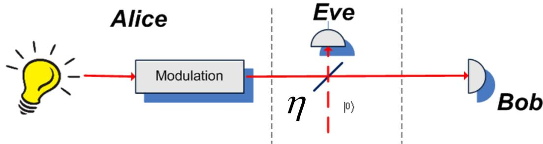
Correlation of the outputs of a beamsplitter:  $C_{BE} \propto V_S - V_E = (V + \sigma) - 1 = 0$
