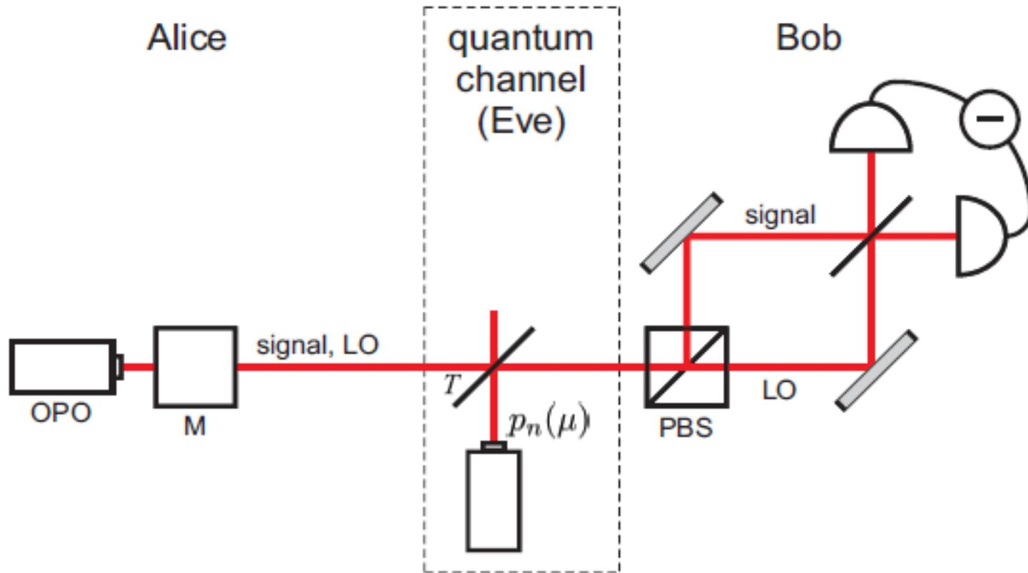
Typical noise model used in CV QKD and parametrized by a mean photon number
