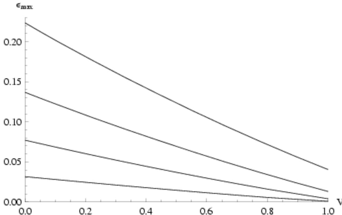
Maximum tolerable versus signal squeezing noise upon limited post-processing efficiency (from top to bottom:  $\beta = 0.8, 0.6, 0.4, 0.2$ )
