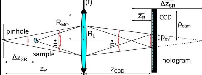
**Hologram** created by interference of divergent reference wave (wavefront radius  $\bar{z}_R$ ) and convergent signal wave (wavefront radius  $\bar{z}_S$ ), originating from the pinhole and the point scatterer of the sample and transformed by a lens with the focal length  $f$ .
