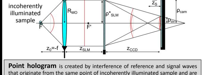
**Point hologram** is created by interference of reference and signal waves that originate from the same point of incoherently illuminated sample and are obtained by splitting the single wave by a Spatial Light Modulator (SLM).
