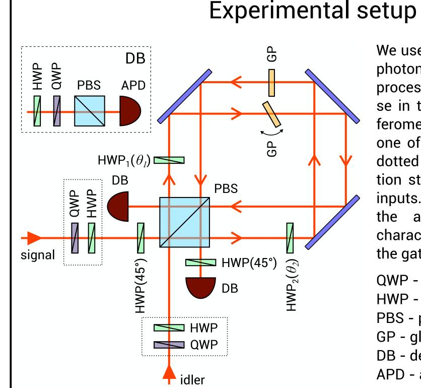
We used source of time-correlated photon pairs generated by SPDC process. The interferometric phase in the displaced Sagnac interferometer was controlled by tilting one of the glass plates (GP). The dotted boxes represent preparation stages for encoding different inputs. The dashed box represents the analysis stages (DB) for characterizing the output states of the gate.
