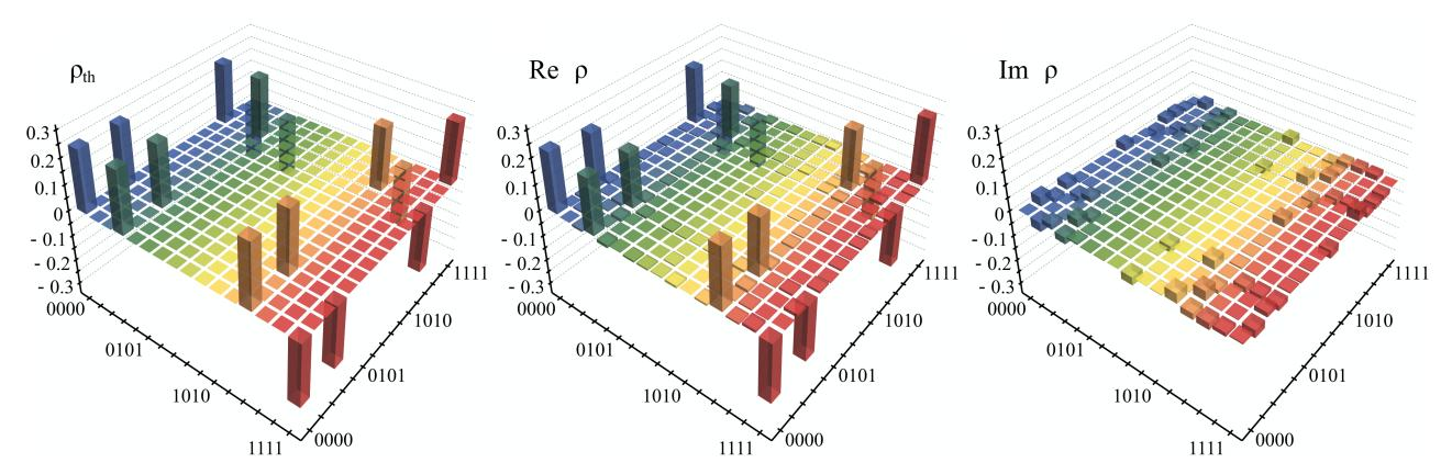
Numerically simulated fidelity of the output states converted from the realistic linear cluster state, where operational fidelity measures the overlap between the realistic state transformed by the experimental conversion gate and the ideal theoretical conversion gate. The total fidelity measures the overall fidelity between the realistic state transformed by the experimental conversion gate and the ideal state transformed by the ideal theoretical conversion gate.
