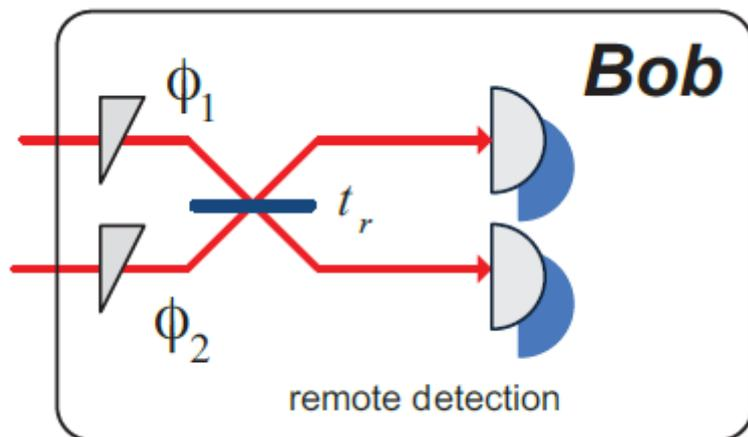
Phase shifts and linear coupling prior to detection on the remote side.
