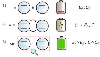
Figure 1: Protocol of charging a battery, represented by a pair of qubits A and B. In the first stage we have two independent copies of qubits with an initial energy. An interaction (coherence) between them is created (stage 2). The third and final step is a detection, which in case of success, increases the energy of the qubits, therefore, charging our battery. The coherence is also increased for some range of parameters.
