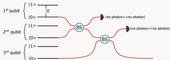
Figure 2: Schematic representation of the charging process for a battery consisting of 3 qubits, inspired by the experimental setup in [3]. The lower energy states are mixed with the help of beam splitters. One of the outputs of BS is used for the detection, the other is sent as the input for the further BS. The projective measurement (detection) is successful when no photon is detected.
