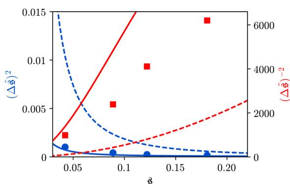
Experimental variances of the separation estimator (blue dots) compared with the direct detection (blue broken line) and the signum-enhanced limit (solid blue line). The latter is corrected for the finite pixel size of  $7.6 \mu\text{m}$ . For completeness, the reciprocal of the variances, called the precisions, are shown in red.
