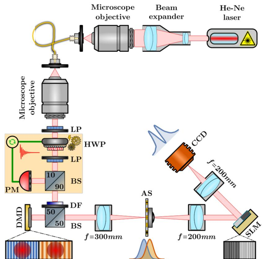
DMD: digital micromirror chip, AS: aperture stop at the Fourier plane of the lens, SLM: spatial light modulator, LP: linear polarizer, HWP: half-wave plate, PM: power meter, DF: density filter and BS: beam-splitter.
