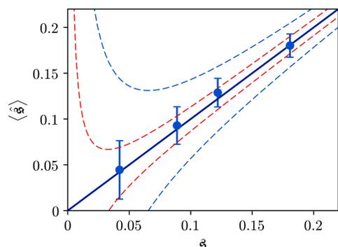
Estimation of the separation from signum-enhanced imaging. Estimator means (dots) and standard deviations (error bars) are shown. Same statistics is provided for the best unbiased estimators from direct (blue lines) and signum-enhanced (red lines) imaging as given by the CRLB. The latter takes in account the finite pixel size used in the experiment.
